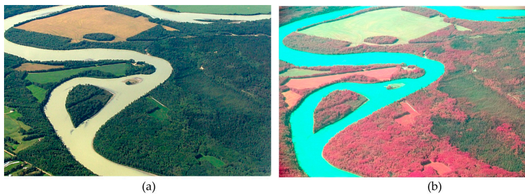
Figure 14. Low oblique images taken about 20 s apart with a Sony DSC-H3 typical RGB digital camera (a) and the Sigma SD1 in full spectrum mode and using the Berkeley 62 mm green X1 filter. Distinction between coniferous and deciduous tree stands is noticeable. The river has a yellowish hue (high sediment load) in (a) and is rendered in a light cyan in (b) as would have been expected from the traditional Kodak CIR film. The images are of the Athabasca River at location 54.44N, 114.47W. Exposure data is: (a) f/8, 1/160 s., ISO125, WB = 5600 K; (b) = f/5.6, 1/160 s, ISO400, WB = 4100 K.
