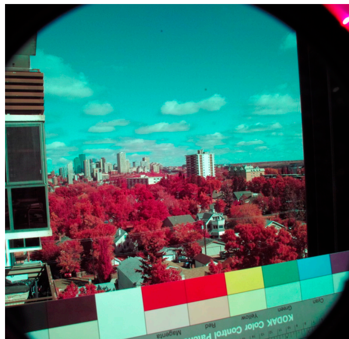
Figure 7. The Izumar 58 mm X1 filter image compensated (calibrated) with a 15 M CC filter. The 5 R was not added. Exposure data is: f/16 , 1/50 s, ISO400, 4100 K.
