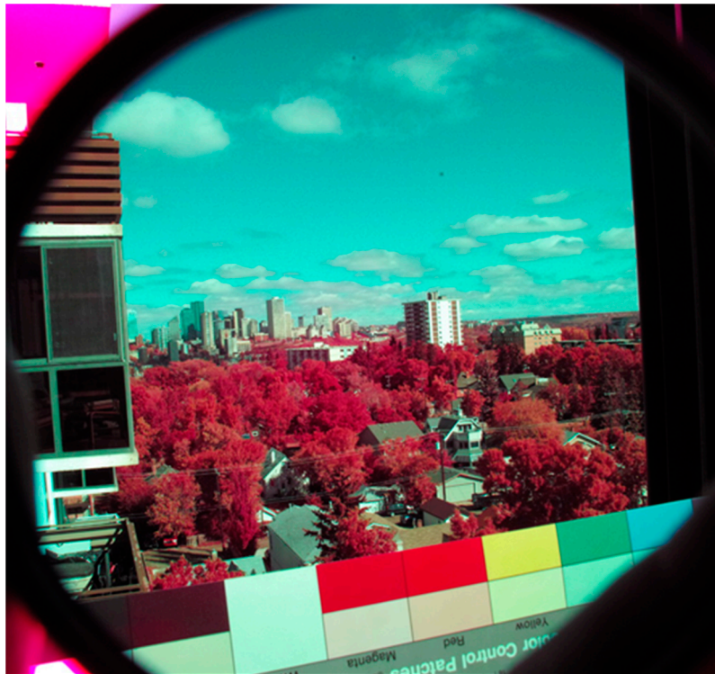
Figure 5. The reference image produced with the Hoya 49 mm X1 filter (H49X1). Exposure data is: f/16, 1/80 s, ISO400, 4100 K.
