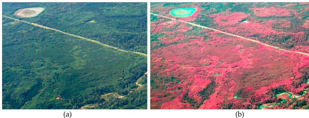
Figure 15. Low oblique true color RGB (a) and Foveon/green-pass (b) images of an area of mixed-wood Boreal forest north-central Alberta, Canada. Acquisition conditions are the same as in Figure 14. The range of hues rendered in (b) make the Foveon/green-pass filter technique well suited for forest image interpretation. The image location is 54.48N, 114.48W. Exposure data is: (a) f/8, 1/100 s, ISO125, WB = 5600 K; (b) f/5.6, 1/160 s, ISO400, WB = 4100 K.
